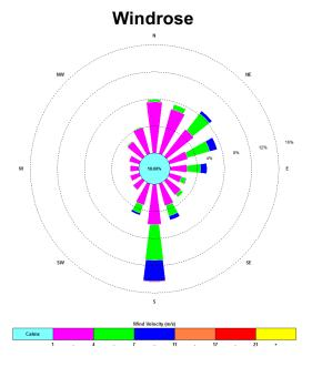
Diagram showing wind speeds and frequencies. The dominant wind direction for October 2018 is from the south. The most frequent recorded high wind speeds are also from the south.
