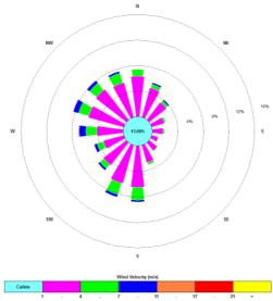
Diagram showing wind speeds and frequencies. The dominant wind directions for June 2016 are from the south, south-south-west and the west-north-west. The most frequent recorded high wind speeds are from the west.
